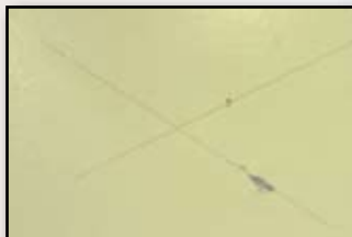
Galvanite™ cold rolled sheet steel with our powder coat finish after a 336 hour salt spray test.
